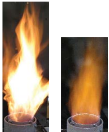
Fuel 100% Water 50vol% Fig.2 Burner flame
