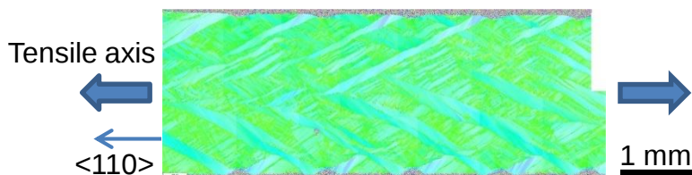
Fig. 2 SEM/EBSD orientation map of Cu single crystal deformed in tension (25%).
