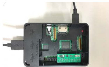
Seismometer on a Single-Board Processor
