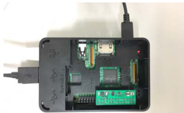
Seismometer on a Single-Board Processor
