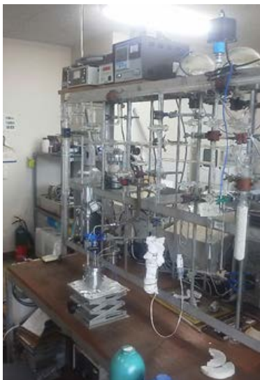
Fig. 1 Volumetric apparatus for measurement of adsorption & desorption velocity of water on adsorbents..
