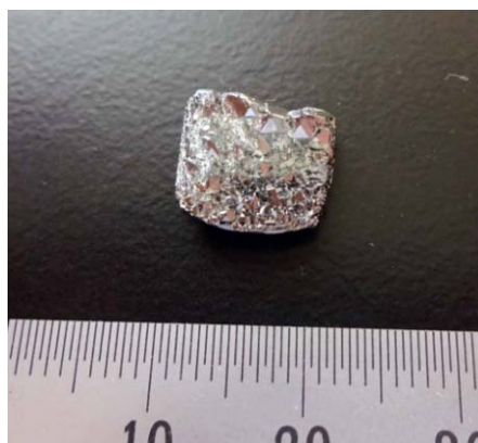
Fig.2. High-pressure reactor Fig.3. Crystal of FeGa 3
