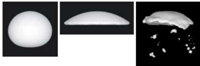
Fig. 1 Bubble motion rising in viscous liquids.
