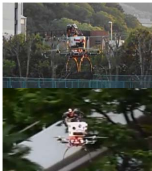
Multicopter Operation by COG Shift
