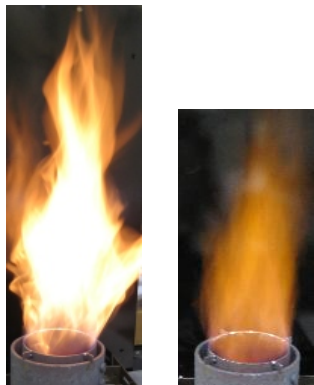
Fuel100% Water 50vol% Fig.2 Burner flame
