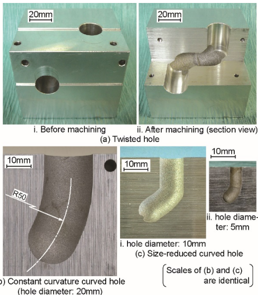
Fig.2 Examples of curved holes machined in this study
