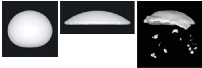
Fig. 1 Bubble motion rising in viscous liquids.
