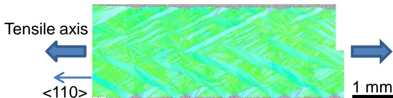
Fig. 2 SEM/EBSD orientation map of Cu single crystal deformed in tension (25%).
