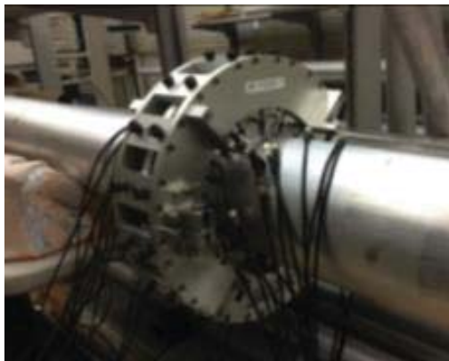
FIG. 2 Piezoelectric guided wave sensor system for piping inspection
