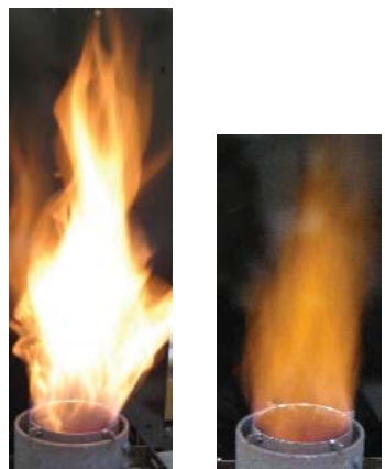
Fuel 100% Water 50vol% Fig.2 Burner flame
