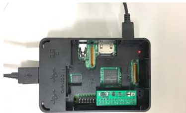
Seismometer on a Single-Board Processor
