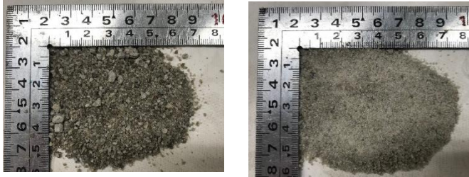
Fig.1 Blast furnace slag sand used (BFS5(left)and BFS1.2(right))
