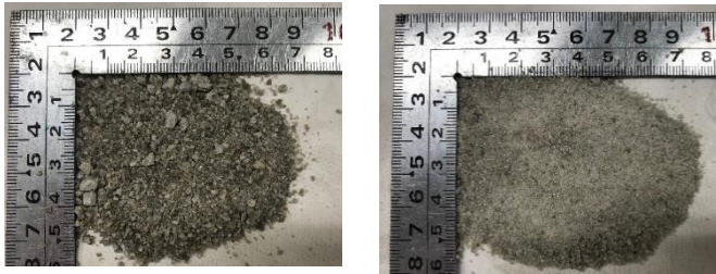
Fig.1 Blast furnace slag sand used (BFS5(left)and BFS1.2(right))
