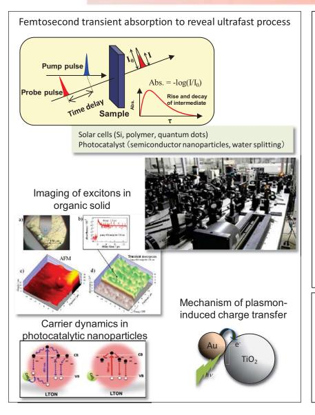
Time resolved spectroscopic systems are developed using ultrafast lasers with pulse duration of ~100 fs.
