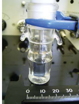
Fig.1 Electrodeposition of PT films on ITO electrodes.
