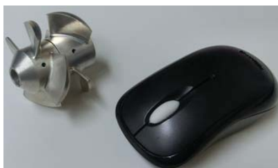
Fig.2 Contra-rotating Small Hydro Turbine
