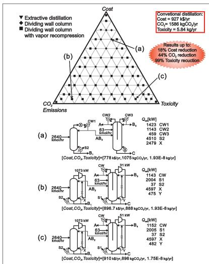
Fig 1. Set of optimal solutions with minimum cost,  ${\rm CO_2}$  emissions and toxicity to humans
